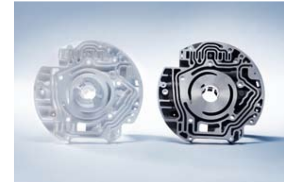
Cover pump (foam model and casting)
